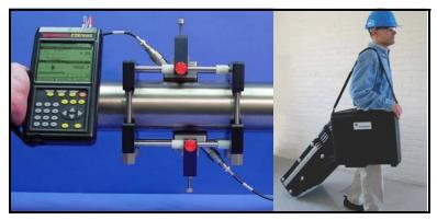
Figure 1-1: PT878GC in Use and in Transport
